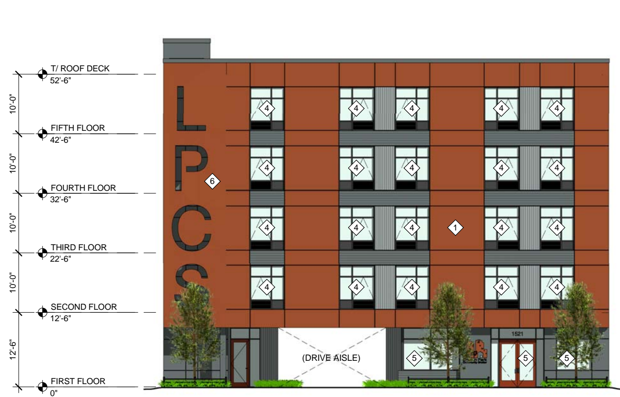
WEST ELEVATION @ STREET METAL PANEL FACADE AREA: 2,580 SF GLASS FACADE AREA: 1,350 SF
