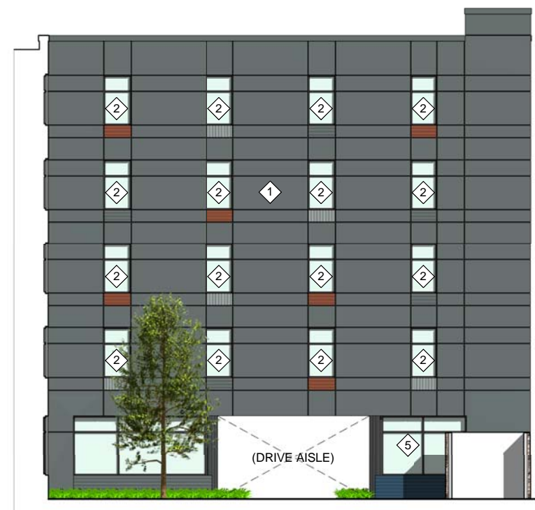
EAST ELEVATION @ COURTYARD METAL PANEL FACADE AREA: 2,440 SF GLASS FACADE AREA: 530 SF
