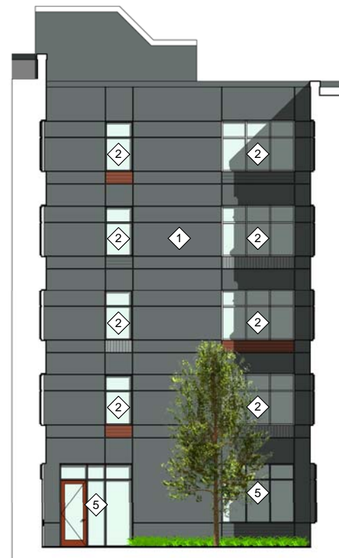
NORTH ELEVATION @ COURTYARD METAL PANEL FACADE AREA: 1,490 SF GLASS FACADE AREA: 450 SF
